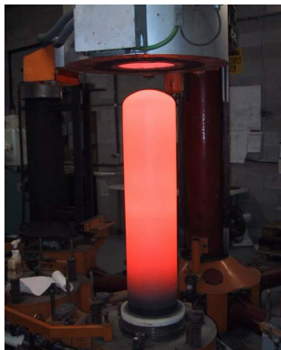
Fig. 4 Reactor chamber for CVD process
