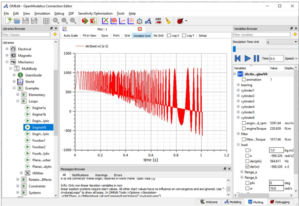
**Figure 1.** OpenModelica simulation of the V6Engine model with 11000 equations. Plotting simulation results using OMEdit. *Left:* Model browser. *Right:* Plot variable browser. *Bottom:* message browser window.
