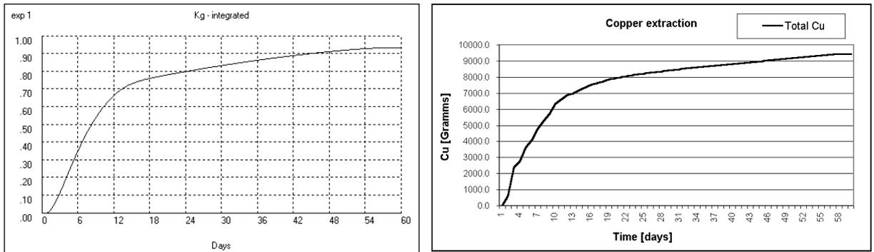
Figure 6. Simulated (left) and experimental copper extraction curves
