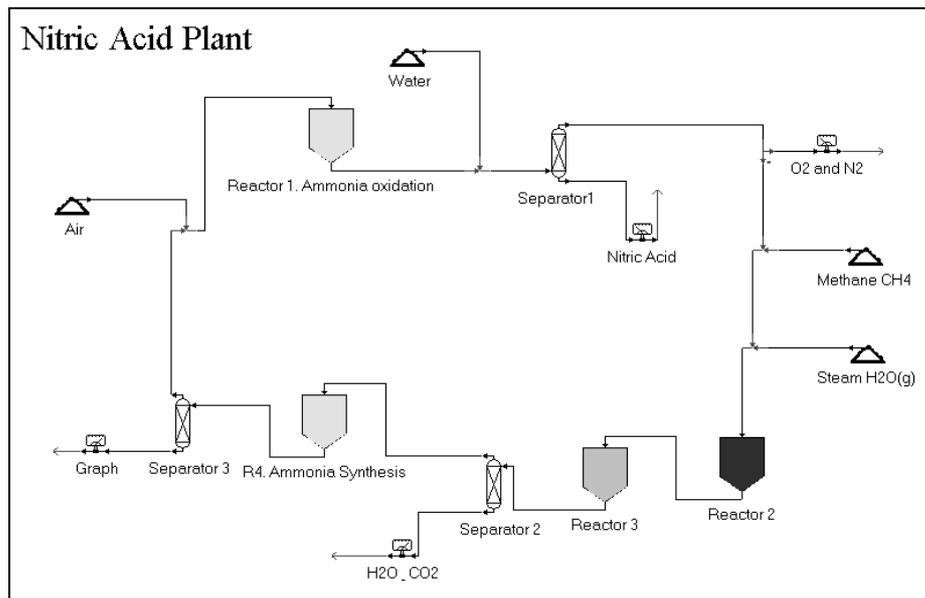
Figure 2. Flowsheet of the nitric acid production process
