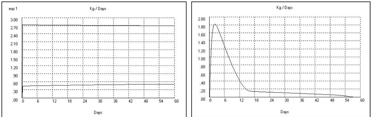
Figure 5. Simulated percolation rate and CuSO<sub>4</sub> content of the PLS
