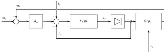
Fig. 6. Block diagram of the voltage sag ride-through algorithm.
