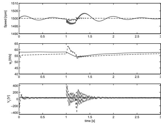
Fig. 7. Simulation of a voltage sag to 70% remaining voltage for a synchronous machine with damper windings, showing the speed (upper graph), flux (middle) and field voltage (bottom) with constant field voltage (solid) and the proposed algorithm (dashed).
