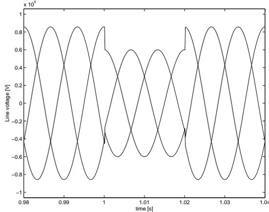
Fig. 1. A 20 ms, 3-phase voltage sag to 70% remaining voltage at 1 s.
