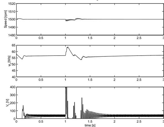
Fig. 9. Simulation of a voltage sag to 70% remaining voltage for a synchronous machine with damper windings with a brush less feeder, showing the speed (upper graph), flux (middle) and field voltage (bottom) with constant field voltage (solid) and the proposed algorithm (dashed).
