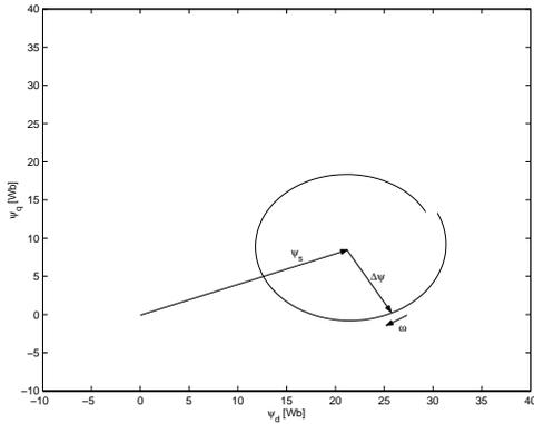
Fig. 2. Stator flux for a 20 ms voltage sag to 70%, showing the first 20 ms.
