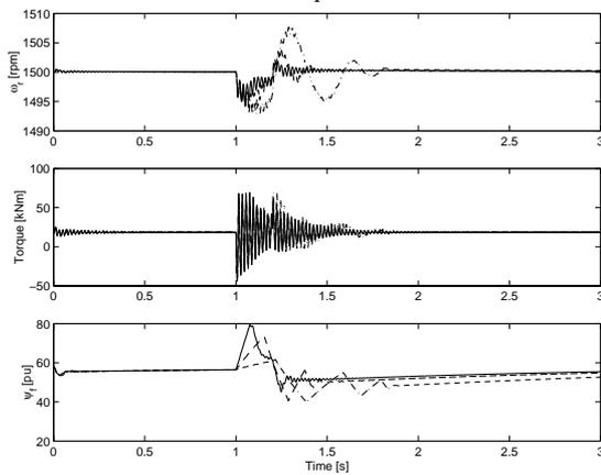
Fig. 11. Simulation of a voltage sag to 50 % remaining voltage for 200 ms for the proposed algorithm, showing machine speed (upper), electrical torque (middle) and  $\psi_f$  (lower), for voltage restriction of 400 V (full), 200 V (dashed) and 100 V (dash-dotted).
