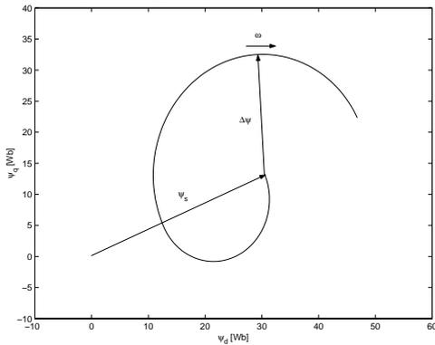
Fig. 5. Stator flux for a 10 ms voltage sag to 70%, showing the first 20 ms.
