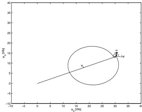
Fig. 3. Stator flux for a 20 ms voltage sag to 70%, showing the first 30 ms.
