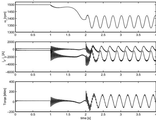
Fig. 12. Simulation of a voltage sag to 20 % remaining voltage for 1s for the proposed algorithm, showing machine speed (upper), stator currents (middle) and electrical torque (lower).
