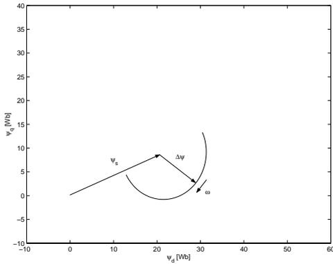
Fig. 4. Stator flux for a 10 ms voltage sag to 70%, showing the first 10 ms.
