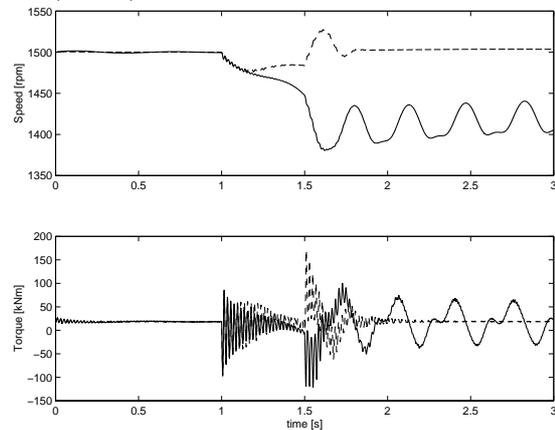
Fig. 8. Simulation of a voltage sag to 20 % remaining voltage for 500 ms for the proposed algorithm (dashed) and with a constant field voltage (solid). The top figure shows the speed and the bottom figure shows the electrical torque.
