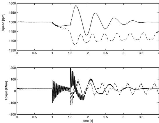
Fig. 10. Simulation of a voltage sag to 20 % remaining voltage for 500 ms for the proposed algorithm (dashed) and with a constant field voltage (solid), concerning an EESM with a brush less feeder. The top figure shows the speed and the bottom figure shows the electrical torque.
