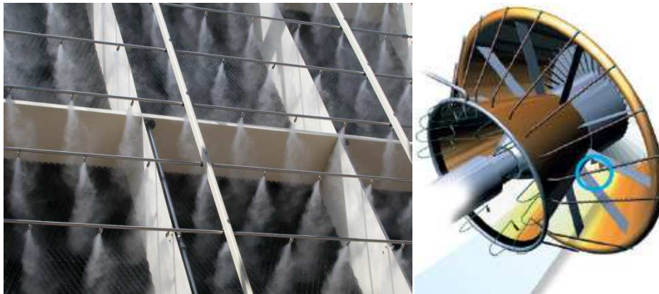
Figure 8. Upstream fog system
