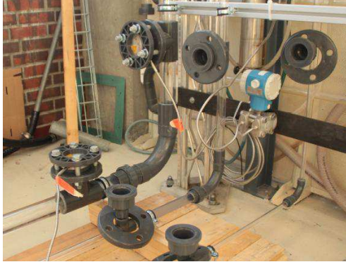
Figure 5 Experimental setup using DP sensors with diaphragm seals. From Krogsæter, 2013.
